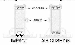
Impacting units provide the most force, but also produce higher noise levels. Air Cushioned (nonimpacting) models feature lower noise levels, but produce less force. When replacing an Impacting unit with an Air Cushioned, it may be necessary to use a larger model, or additional vibrators to achieve proper material flow.
